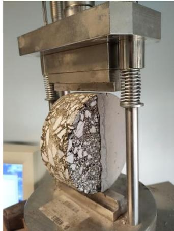
**Figure 7. ITS set up for MMT sample.**
