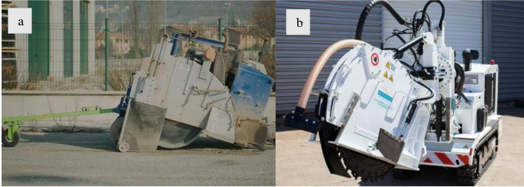
**Figure 1. Sawing machine used for micro-trenching (a) and mini-trenching applications (b).**
